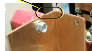
Phase detection wire must be in this orientation
