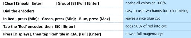
The Parameter tiles in the CIA remap based on the channel or fixture type selected.
