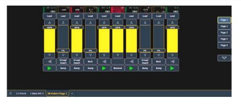
Remember that a single page of faders is a bank of 10. So a single page of faders is shown by default. On the right of the display are page buttons to navigate to other pages. The faders themselves behave just like physical faders.
