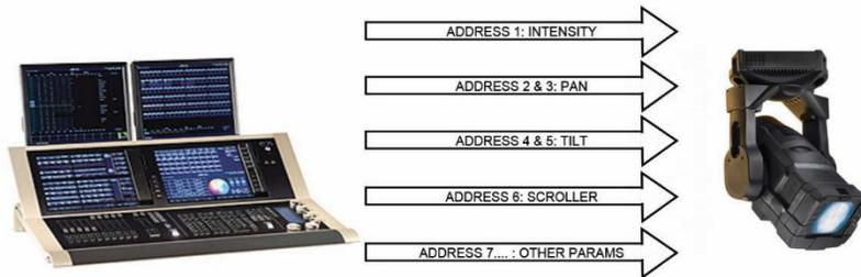
Each motor that is associated with a parameter listens to its own DMX address – move the DMX value, move the motor.
