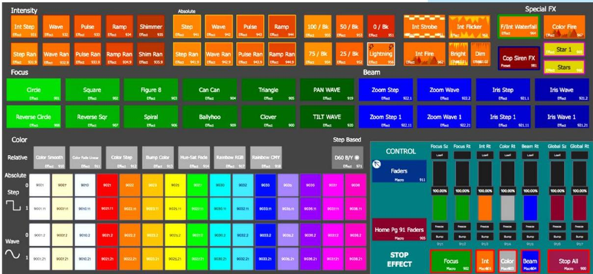
This is an example of a magic sheet laid out for effects. It is divided into parameter type, so the user can easily find what kind of effect they are looking for. There are relative & absolute effects mixed in. There is only one step-based effect just to have an example. Step based effects are most often show specific, and therefore are not typically included in a library page.
