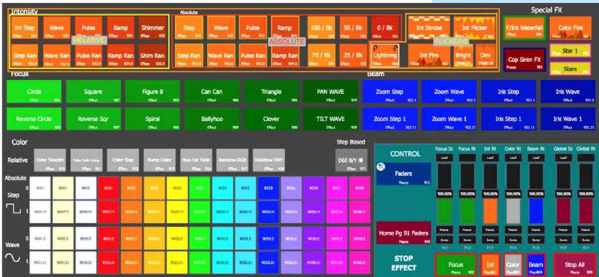
The orange buttons on top are intensity effects. They are orange for consistency and organization...the console color for intensity palettes is orange. They are divided into 3 sections
