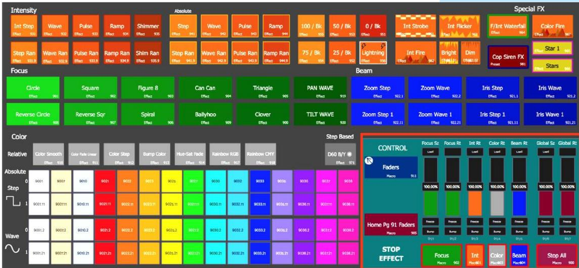
This last section on the bottom left is a control section to control running effects. It contains virtual faders that are set to global effects rate & size. They are divided by color to show which type of effect they are filtered to. There is also an overall global effects override.
