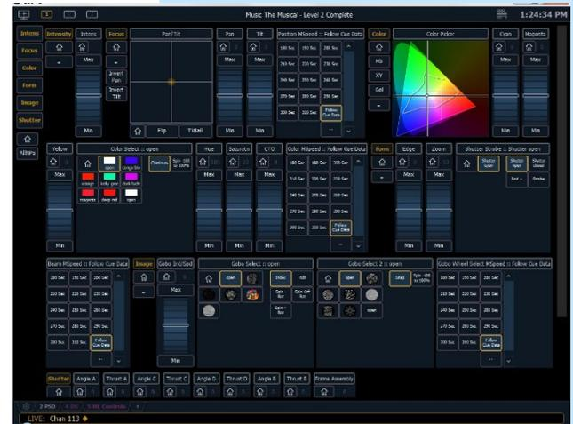
The parameters displayed will change based on the device(s) selected. If multiple fixture types are selected, all parameters combined are shown.
