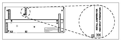
Figure #2: Backplane of CMEd Save these jumpers to send back with the loaner processor.
