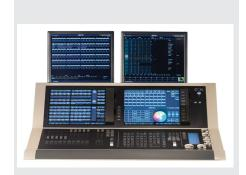
The Eos family of consoles, including Element, Ion, and Eos, handle dimmers, LEDs, and moving lights in a way that is different than legacy consoles. Understanding how it defines channels and handles DMX addresses is important in determining which console is right for the venue.
