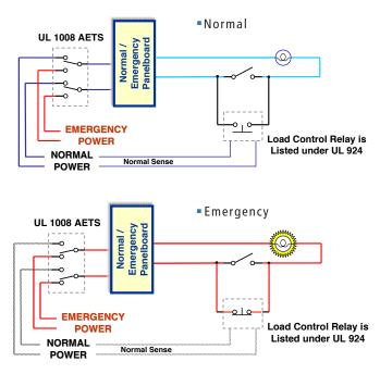
Case 3—Normal/emergency lights on switches or wall-box dimmers
