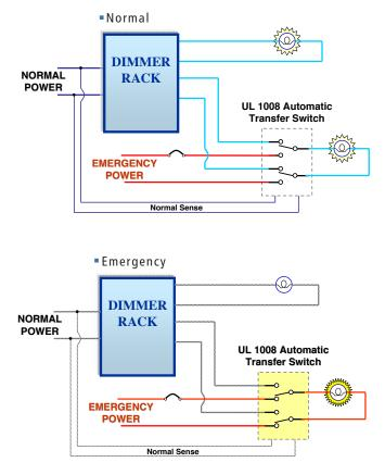
Case 5—Normal/emergency lights on a UL 1008 branch circuit automatic (emergency) transfer switch
