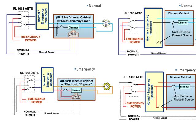
Case 4—Normal/emergency lights on a UL 924-Listed dimmer rack or relay cabinet
