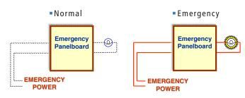
Case 1—Emergency-only lights on an emergency-only circuit
