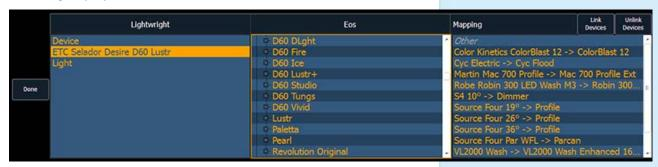
The text fields in the Patch display and database will rename based off of the Lightwright imported fields. The link will appear in the Mapping column. To unlink a device, select it from the Mapping column, and then press **{Unlink Device}**.
